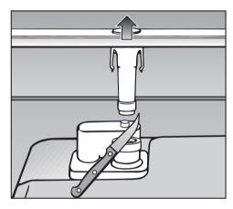
■ Cut off the vent cap located at the right rear of the triple filter system, as illustrated.
